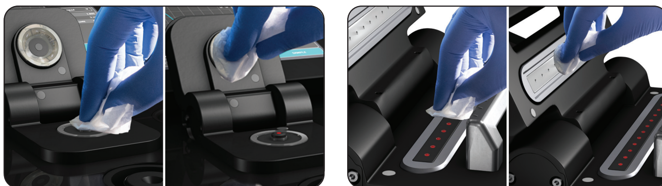
Figure 1: The Pedestal and mirror of the NanoPhotometer® are being cleaned with a lint-free tissue.
